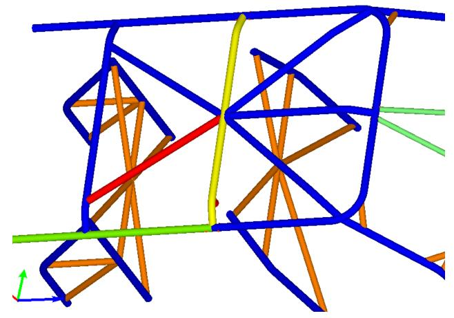
Due to increase requests all intersecting tubes has been made as fully overlapping nodes. This means identically mirrored parts will have different notches to overlap the other tube. **ALL JOINTS SHOULD BE FULLY WELDED!!** We don't recommend welding only the visible joints. Tubes must be ALL fit together and then disassembled and welded in sequence to ensure full strength.
