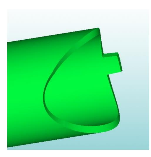
Slot and tab cuts will locate the parts with these features.
