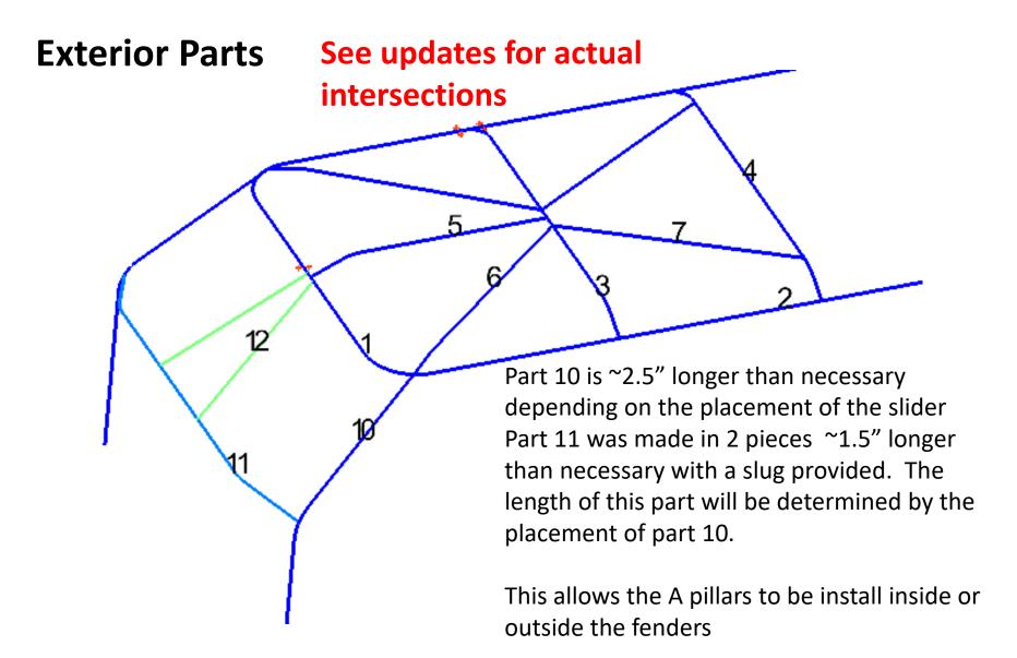
For visualization the parts are shown as centerlines only Part Numbers engraved within 3" of the end of part Passenger side parts are followed with a M (for Mirrored)
