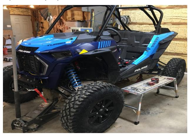
Even with proper support the factory cage will spring out of alignment depending on the condition of the machine as well as factory tolerances. Yes this is a RZR shown but the same principal applies
