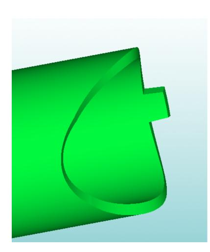
Slot and tab cuts will locate the parts with these features.
