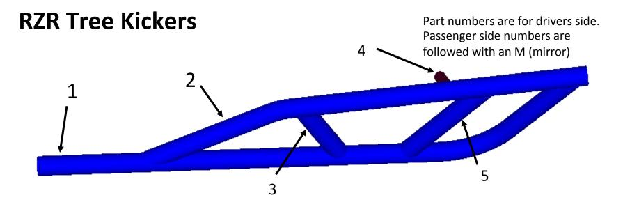
We start assembly by welding Part 4 to the upper tab on the bench. The tube should be centered on the lower hole and perpendicular to the tab.
